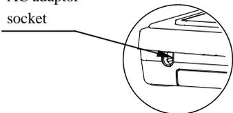
Plug the AC adaptor to the AC adaptor socket on the side. The AC input requirement could be 100,120,220,230 or 240Volts (50/60Hz) depending on the area where used, so please verify that the adaptor is correct
